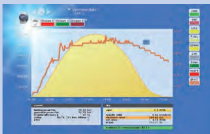
Daily curve with ambient temperature sensor
