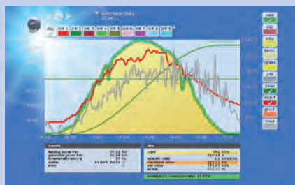
Daily curve with solarization sensor (green), wind sensor (grey), module temperature (red) and yield curve (yellow)
