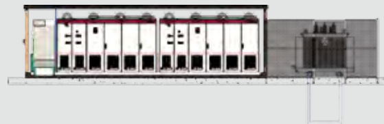
Scheme with two inverters with Multi-MPPT configuration (also available with Master-Slave or Monoblock configuration) 2 x 1,070 kVA
