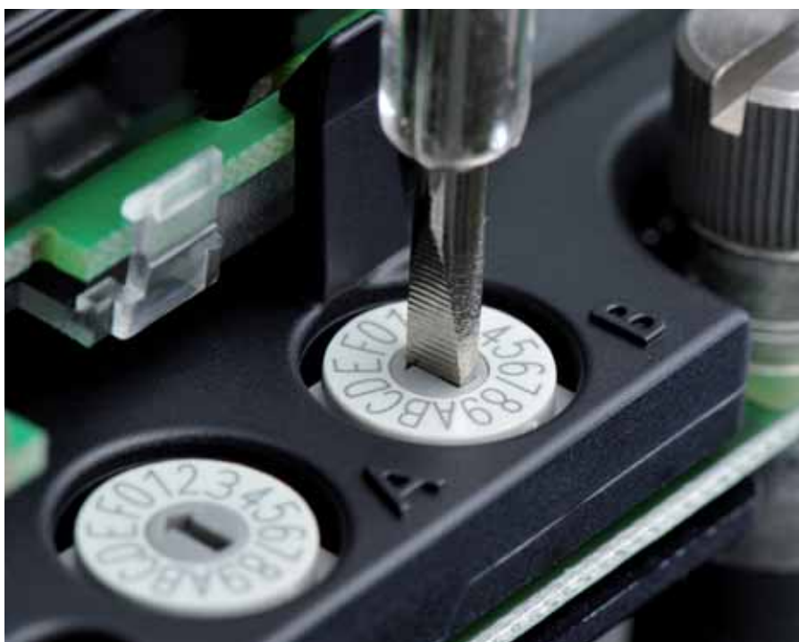
Country-specific configuration in the blink of an eye: rotary switch on the Sunny Boy 5000TL
