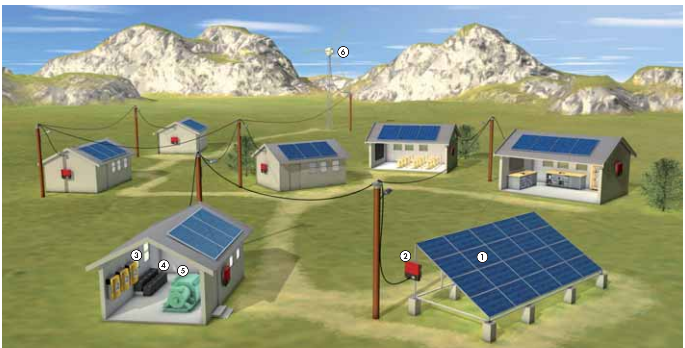
Components: 1. PV array, 2. SUNNY BOY, 3. SUNNY ISLAND, 4. Batteries, 5. Diesel generator, 6. Wind turbine system
